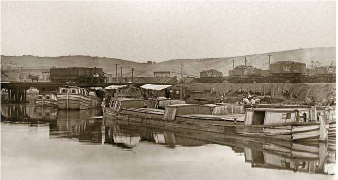
Above: C&O Canal boats waiting to be loaded with coal from Cumberland & Pennsylvania hopper cars.
